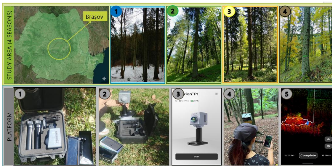
Figure 1. Study Area and the use of FJD Trion Model P1 Platform. Legend: The study area seasons: (1) winter, (2) spring, (3) summer, (4) autumn. The platform: FJD Trion Model P1 scanner (1), scanner assembly (2), scanner App screen (3), scanning with the platform (4), and a scanning process (5).
